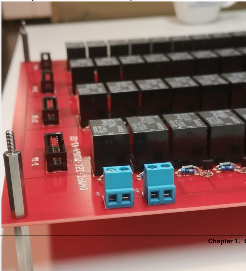
Position 9 spacers above the MUX board, and 9 spacers below
