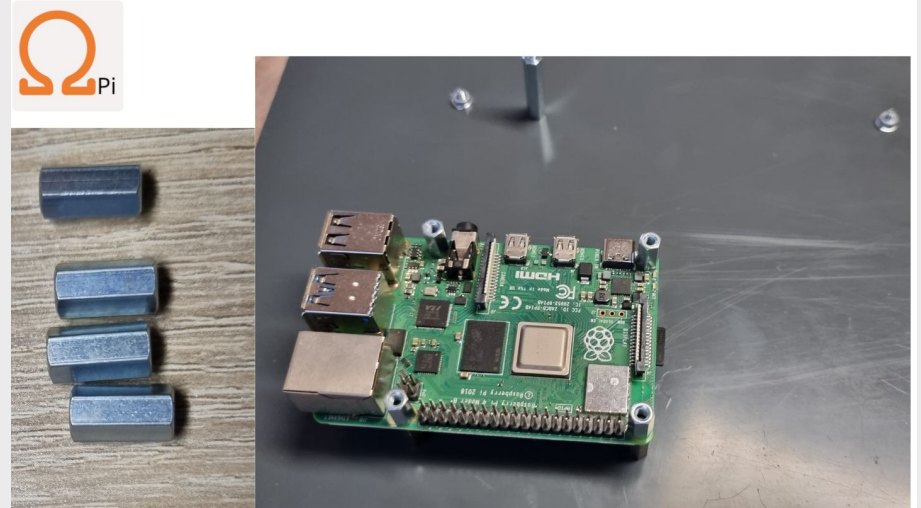
Fit 4 spacers (female/female, M3, 11 mm)
