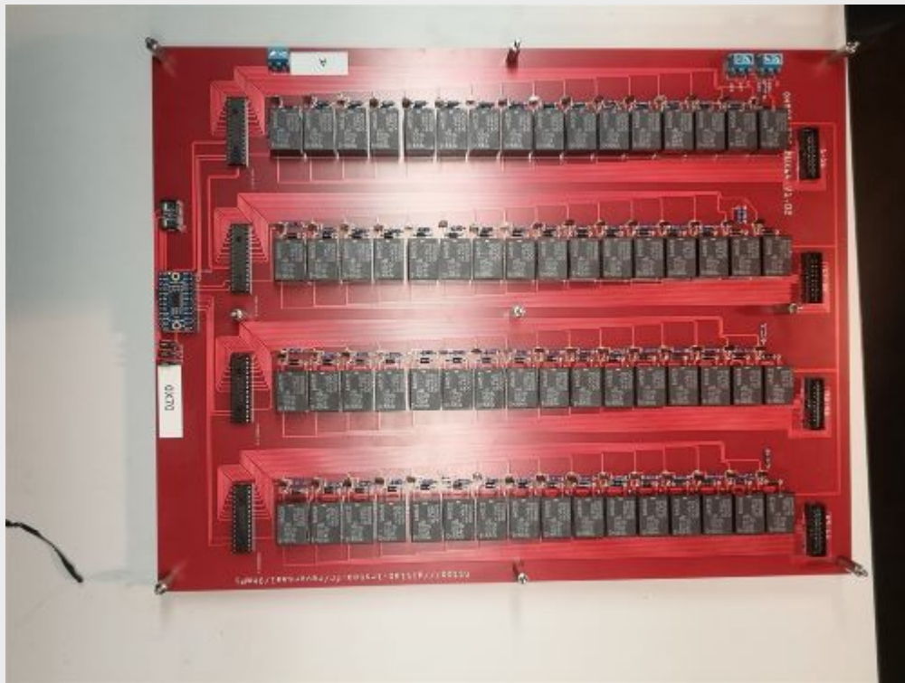
Position 9 spacers above the MUX board, and 9 spacers below
