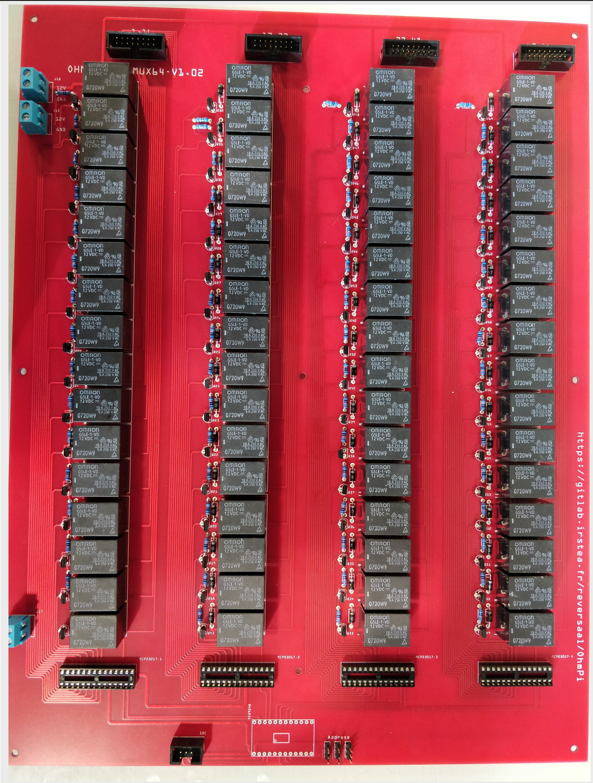
Installation of DIP Dual In Line Socket 2*14
