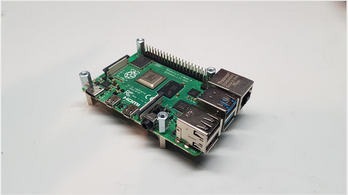
Mounting the upper spacers on the Raspberry Pi (female/female, 11mm, M3)
